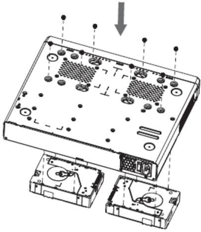
3. Connect the HDD's power and data cables to the device's corresponding ports.
